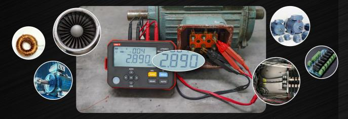
Measuring the resistance of all kinds of wires, switches, connectors, contactors, fuses, coils, transformer windings, metal riveting, and so on.
