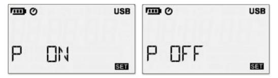
In the auto power-off setup page, press UP or DOWN button to enable or disable Power Off Function.
