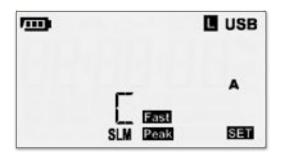
In SLM function setup page, press **RIGHT** and **LEFT** to switch test function. Press **UP** and **DOWN** to switch among settings: Sound level range > Time weighted > Frequency weighted > Peak frequency
